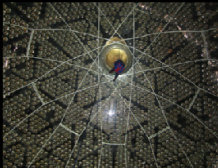
New calibration hardware: light injection system installed
